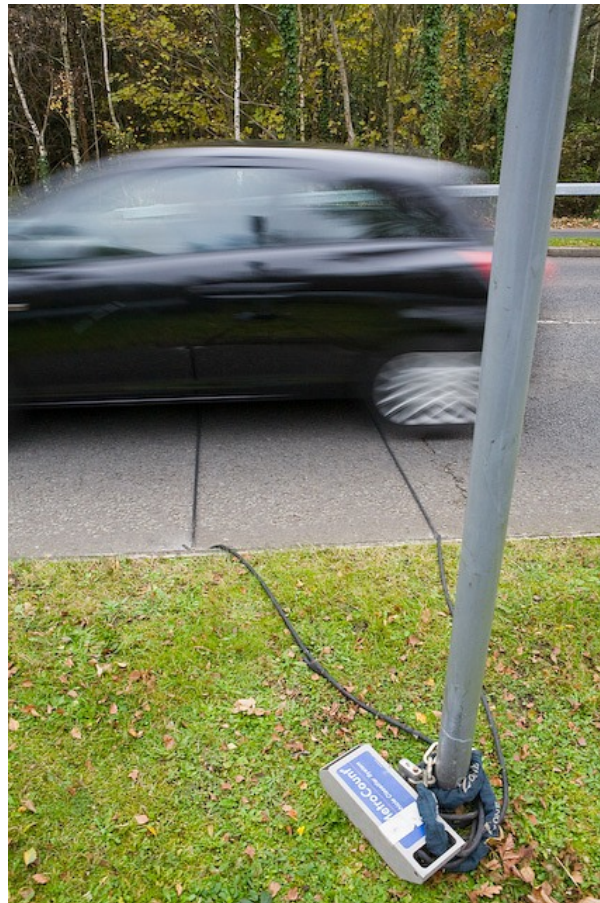
Figure 6: An example of a pneumatic tube traffic counter, installed above the road.
